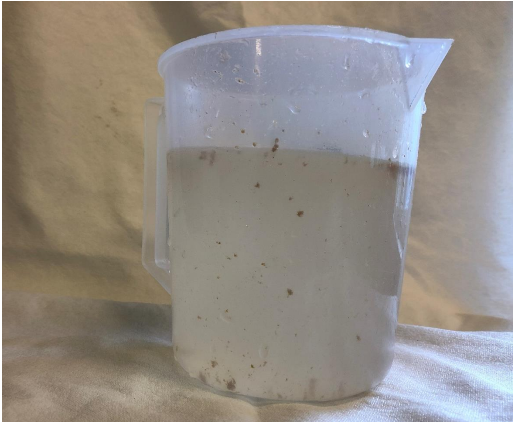
Figure 3. Water V3, water from dewatering belt press.
