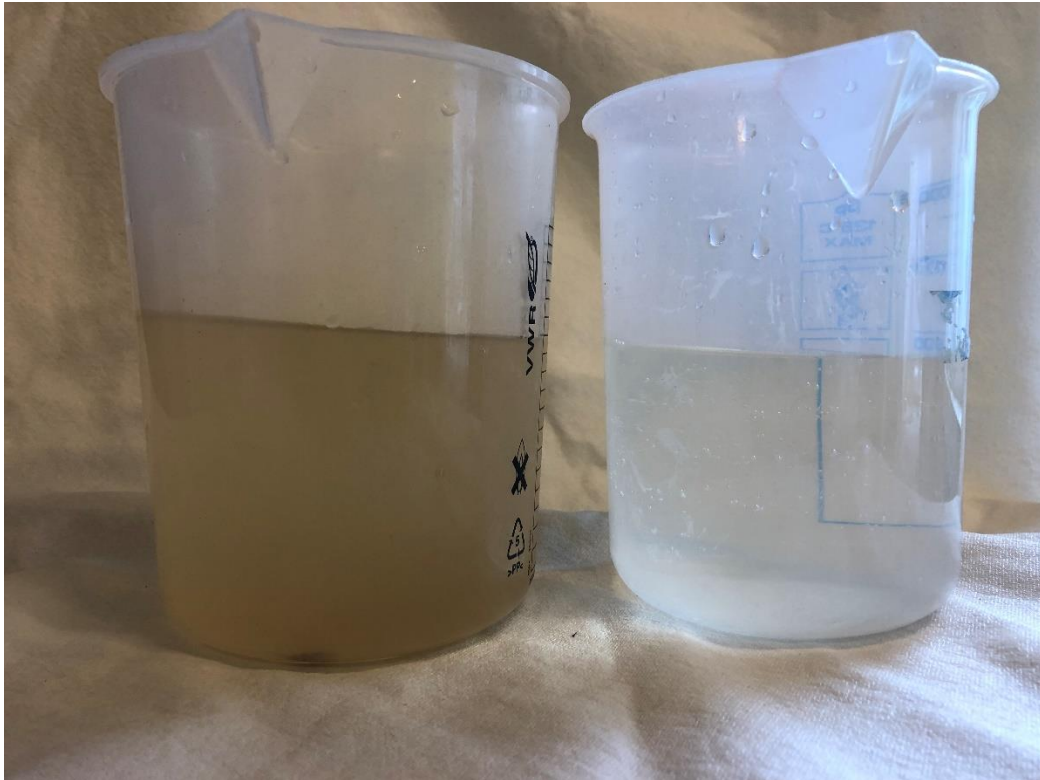
Figure 6. To the left, ingoing V2. To the right, V2 purified in AxoPur using aluminum electrode.
