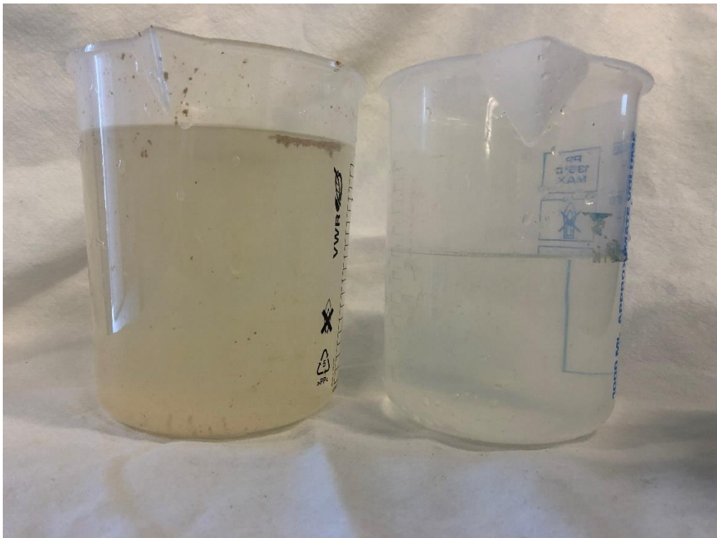
Figure 6. To the left, ingoing V3. To the right, V3 purified in AxoPur using aluminum electrode.
